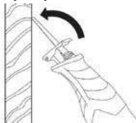
as the blade foot fully lays on the surface of the workpiece, continue sawing alongside the desired cutting line. For certain work, the saw blade can also be inserted turned through by 180° and the sabre saw can be guided accordingly in a reversed manner.
