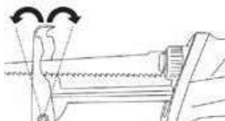
If you need to reduce the cutting capacity of your tool (depth of cut), the pivoting foot plate may be adjusted as follows. Loosen the securing screw on the underside of the front housing with a hex key. Slide the pivoting blade foot to the required position. Tighten the screw and check that the blade foot is firmly latched.
