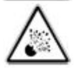
Cylinders containing shielding gasses store them at high pressures. If they suffer some kind of breakdown they can explode. Always treat cylinders with care and weld as far away from them as possible.
