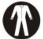
The entire body of the welder is subjected to the possible action of aggressive agents, so it must be fully protected. Wear safety boots, gloves, sleeves, leggings and leather aprons.
