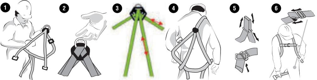
1.- Fully deploy the harness. 2.- Take the harness by the dorsal buckle. 3.- Adjust to the measure of the user by means of the dorsal regulator. 4.- Put on the harness with the regulator and the pickaxe located on the back. 5.- Adjust and fasten the pectoral metal buckles and the plastic buckle. 6.- Adjust and fasten the leg buckles. The harness must be adjusted in such a way that it allows all the movements to be carried out without any impediments.
