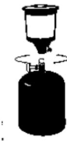
Screw the lamp onto the cylinder and fully tighten.
