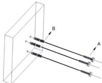
Drill three holes into the wall taking care to measure the distances to fit the base. Insert the three plastic anchors (b) into the holes and then inserting the three heavy-duty screws (A) into the anchors. Use a drill to secure.
