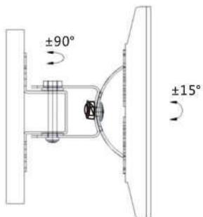
Move the wall plate up and down in the desired direction by using the spanner (H). Once you have the desired angle, tighten the adjustment screws.
