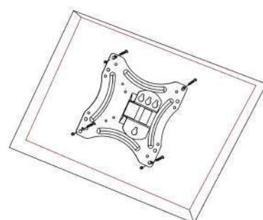
Install the TV to the wall plate by using parts C or D or E that fit your TV the best. The washers (F or G) are provided to ensure a better fit.
