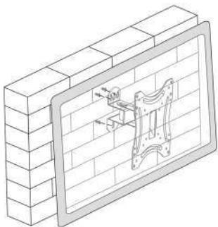
Hang the wall plate onto the heavy-duty screws, be noted that the small head is up side. Then tighten the heavy-duty screws.
