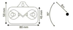
Choose a mount to fix the device. Fix the device at height according to the targeted game:
